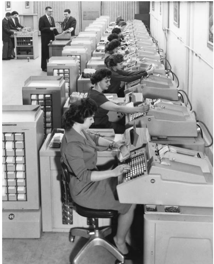
Figure 2. The "information age" coupled computing technologies to the routinized processing of information. Here, in 1960, nine operators enter bank transactions into Burroughs F-600 machines, probably at a St. Louis, Missouri, bank. (Courtesy Charles Babbage Institute.)
